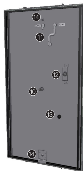
Exploded View 2: Rear View of Filter Access Door
